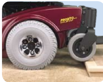
The base of the Pronto M51 flexes to keep all six wheels on the ground at all times for optimum stability.
