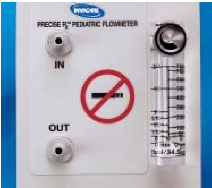
Detail of Invacare PreciseRx pediatric flowmeter.
